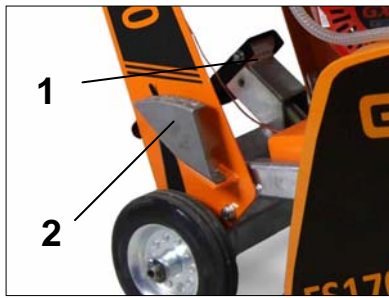
1. Hand wheel - raising and lowering 2. Depth control
